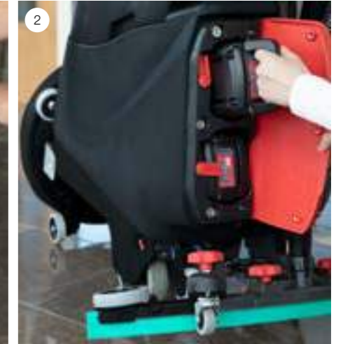
1 TTB1840NX Battery Replacement
