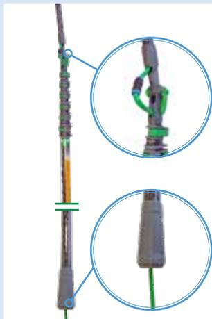
Insert the hose at the bottom of the pole, lead it out at the top, through the angle adapter and connect it there with the quick connector.
